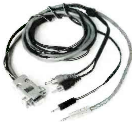
FIG. 4—THE AUTHOR'S CUSTOM CABLE, which is used to connect the Synergy Card to an audio system.
