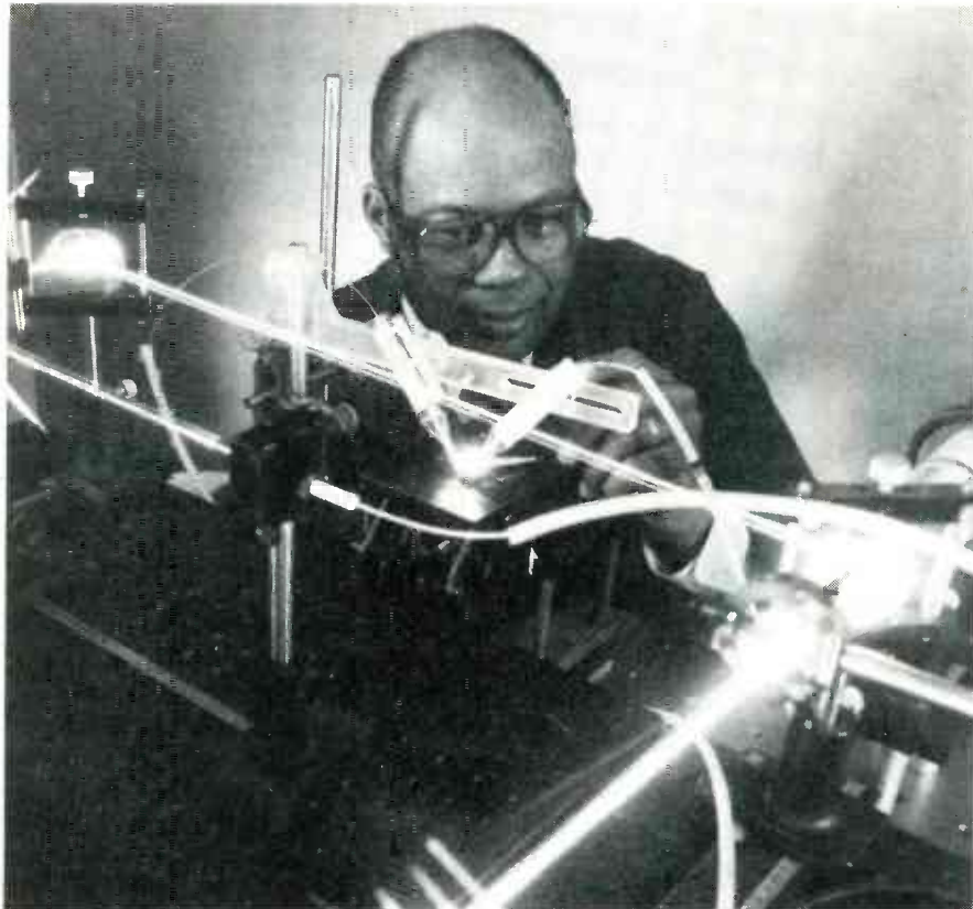
GE ENGINEER DR. RICHARD I. HARTLEY adjusts the flexible tips of a new welding system that carries the power on thin fiber-optic cables and applies the heat to both sides of the weld simultaneously.
